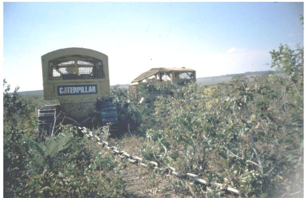
Figure 2.3: Clearing of native cerrado vegetation with the *correntão* chain system © Ulrike Bickel 2003
